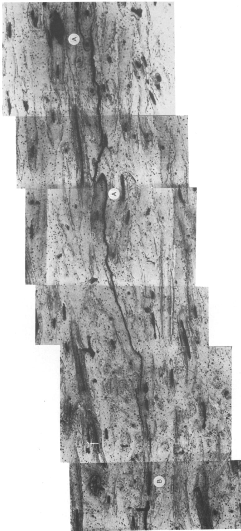
Figure 6 Fracture profile illustrating crack propagation around osteons (A) and crack arrest in a canal (B) ( \times 72 ).
